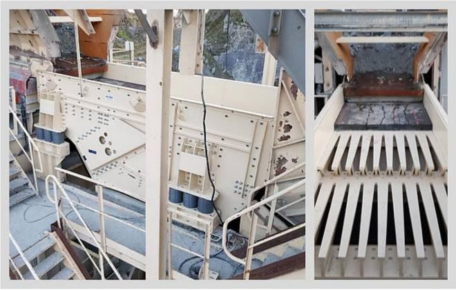
capacity (t/h): 600 | bulk: Rocks | density (t/m<sup>3</sup>): 1,6 | grain size (mm): 0-1000
