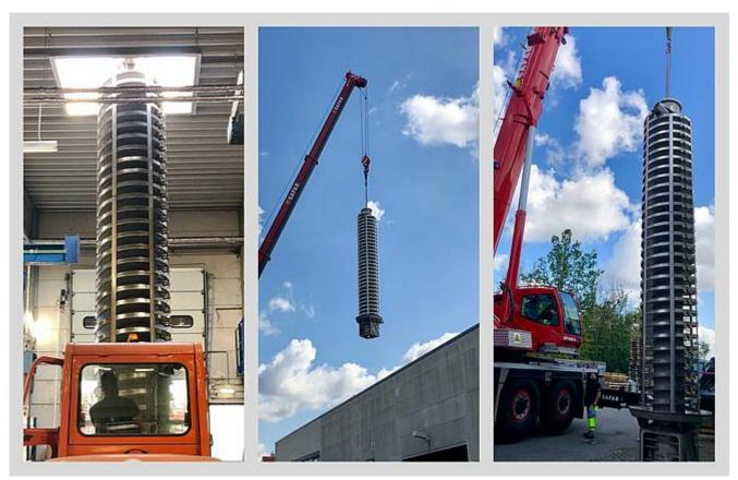
capacity (t/h): 2,2 | bulk: Hot Crunchy cereals | density (t/m³): 0,3 - 0,5 | grain size (mm): 1 - 30
