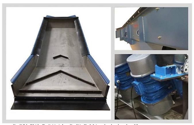
capacity (t/h):  $70 \mid \text{bulk}$ : Kohle | density (t/m³):  $1,1 \mid \text{grain size (mm)}$ : < 10
