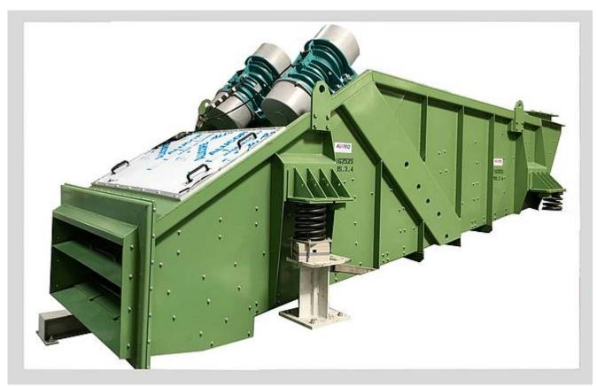
capacity (t/h): 400 | bulk: Limestone | density (t/m³): 1 | grain size (mm): 0 - 80
