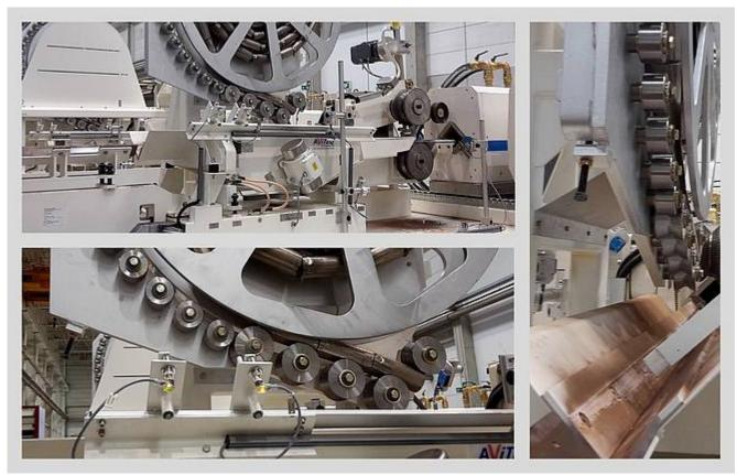
capacity (t/h): 4 | bulk: forging sticks | density (t/m³): Stückgut | grain size (mm): Ø40-110 mm, L=1,5 x Ø bis 600 mm
