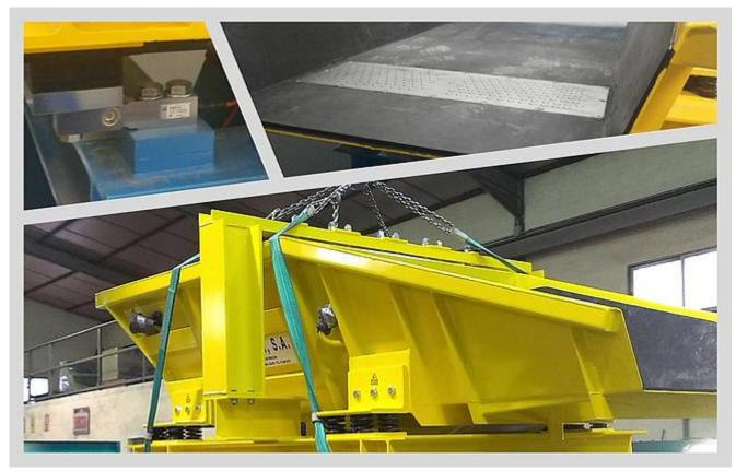
capacity (t/h): 7,2 | bulk: Screws and nuts | density (t/m³): 1,5 - 5 | grain size (mm): M8
