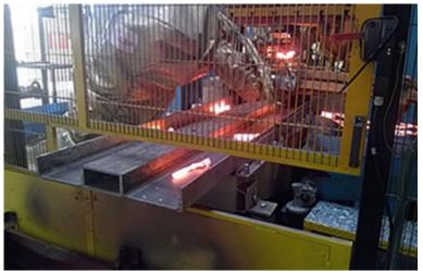
capacity (t/h): 1 Stck. / 6 Sek. | bulk: Forging scrap | density (t/m<sup>3</sup>): 1 | grain size (mm): 350x50x50
