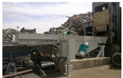
capacity (t/h): 1 Stück / 5 sek. | bulk: Scrap metal | density (t/m<sup>3</sup>): 1 Stück | grain size (mm): 500x500x300
