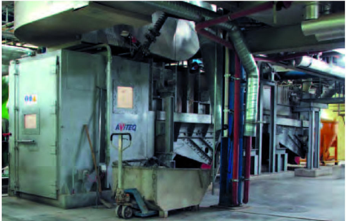
4 ▶ AVITEQ vibrating conveyor for ash processing Eingehauste Vibrorinne von AVITEQ
